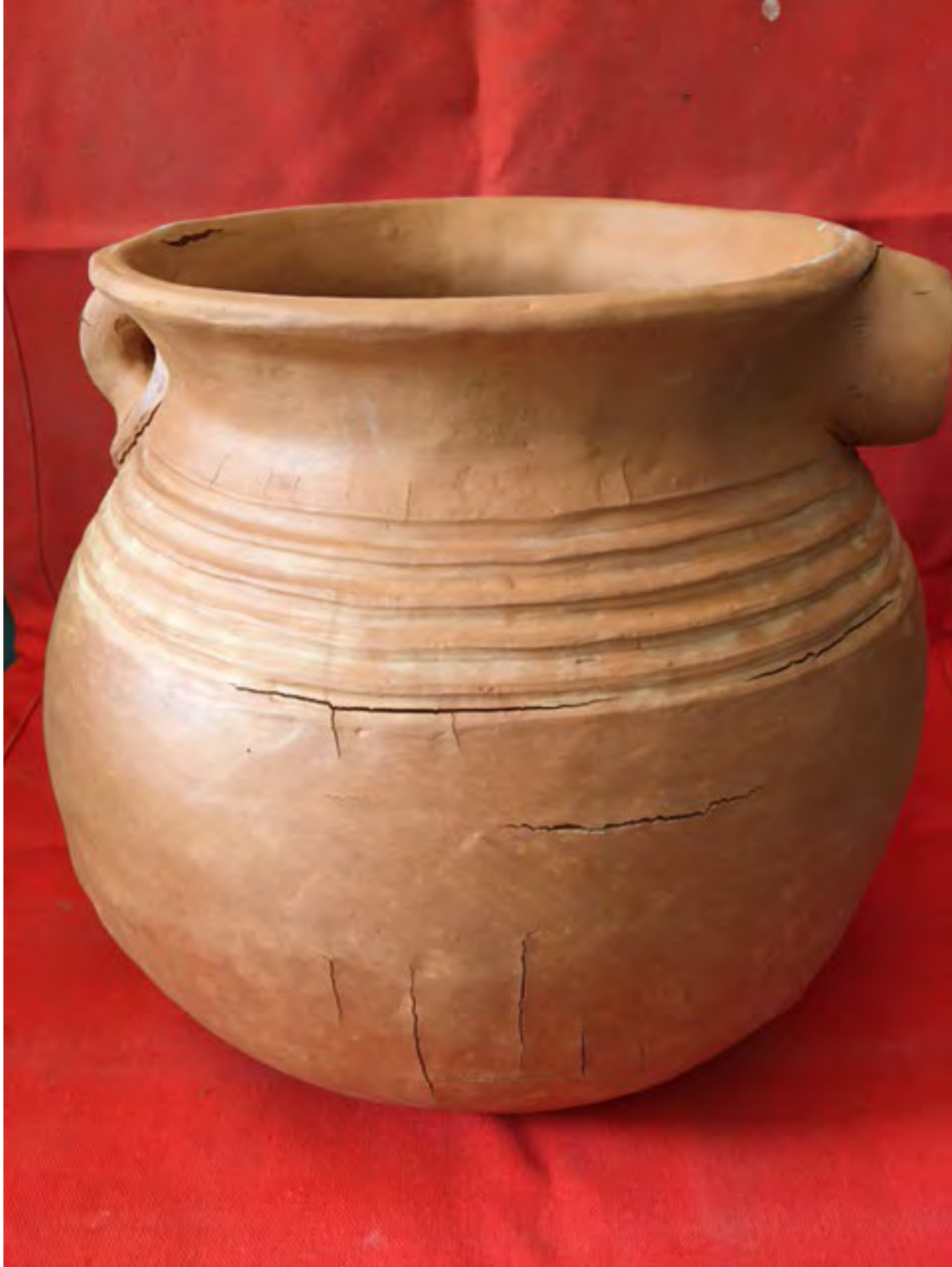
Fig.30. Ipswich ware reproduction pot (Jnana Emmett) showing the way the London clay cracks due to diferential shrinkage between inside and outside - the cracks do not go all the way through. Fired to 950 degrees in an electric kil. This problem was solved by adding more sand.
