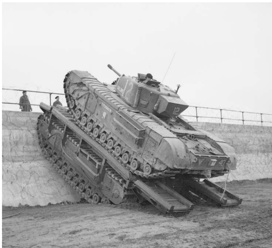
Figure 52. A Churchill 'Ark' of 79 th Armoured Division practising on a concrete anti-tank wall on the Orford training area as part of training before D-Day. (Imperial War Museum, H36593)
